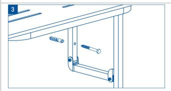
**Fixing:** For timber drill with pilot drill, for concret drill spot marks with 10mm bit. Plug and screw seat to wall using the 304 Stainless Steel M8 x 75mm hexagon coach screws supplied.
