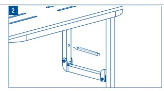
**Positioning:** In the horizontal position, level check and spot mark wall through seat frame mount holes.
