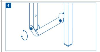
**Checking:** Check seat is firmly secured to wall and Tension Grip Hinge screws are appropriate for ease of movement.
